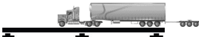
Figure 13: Semitrailer and dolly weighed with dolly off the weighbridge
