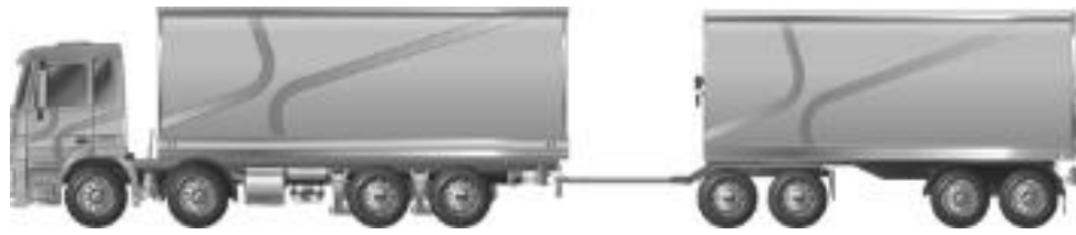
Figure 36: Example twin steer truck (Code 73 – 4 Axle Twin Steer Rigid Truck & 4 Axle Dog Trailer)
